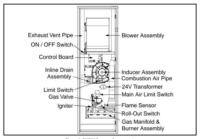
Figure 3. CMF95 Furnace Components
