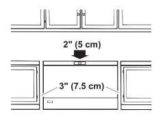
**IMPORTANT:** Do not install the freezer near an oven, radiator or other heat source. Check the strength of the floor before installing your freezer. It should hold the weight of a freezer fully loaded with food.
