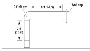
The following example falls within the maximum recommended vent length of 35 ft (10.7 m).
