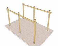
Lift, position and attach the second Post/ Side Girder section to post hardware.
