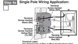
Use Terminal for 3-Way or More Applications Only. For Single-Pole Applications, Do Not Remove This Label.
