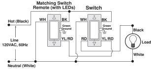
**NOTE:** The switch **must** be installed in a wall box that has a Load connection. The matching remote must be installed in a wall box with a Line Hot connection and a Neutral connection. A Neutral wire to the matching remote needs to be added as shown.
