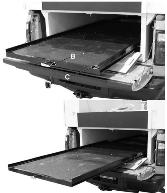
Figure 4-4 – Deck Slide Handle (Deck at First Stop) Figure 4-5 – Deck Slide at Second Stop (Fully Extended)
