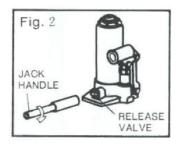
3) Place jack under the vehicle at the proper lifting point. (Refer to Owner's Manual.) If needed, turn the extension screw counterclockwise until it comes into contact with vehicle.
