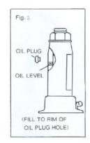
4) Fill with a good grade hydraulic oil only. (Fill to the lower rim of oil fill hole.) Purge system of air as described in this manual.
