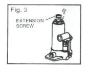
4) Insert jack handle into handle socket. Pump the handle to lift the vehicle to the desired height.
