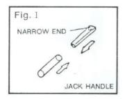
2) With the narrow end of the jack handle, close the release valve tightly by turning it clockwise.
