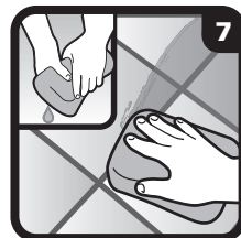
Wait for firm joints Lightly clean off excess grout with sponge. CAUTION: Do Not Over Water.
