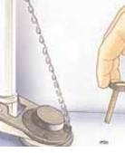
the bolts through the holes with the bolt heads on the inside of the tank.
