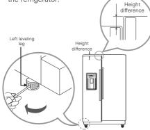
**NOTE:** Having someone push backward against the top of the refrigerator takes some weight off of the leveling legs. This makes it easier to adjust the legs.
