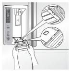
2 To reinstall the tray, slightly tilt the front of the tray and snap the ribs into the holes.
