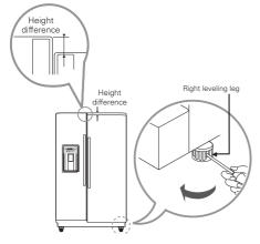
2 Open both doors again and check to make sure that they close easily. If the doors do not close easily, tilt the refrigerator slightly more to the rear by turning both leveling legs counterclockwise. It may take several more turns, and you should turn both leveling legs the same amount.
