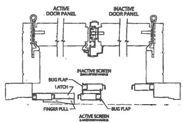
4. Install the jamb strike after closing the screen panel to note the proper location of the of the strike flange. Note the strike flange can be positioned either up or down. Install one screw and test for fit; adjust, install second screw and tighten.
