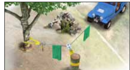
A redirected pull. If there's no straight, clear line to the anchor point, use a pulley block.
