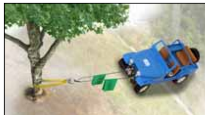
A typical double-line winch and pulley arrangement doubles winch capacity.
