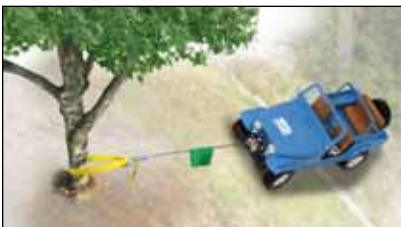
Some typical pulls: a single line straight pull.
