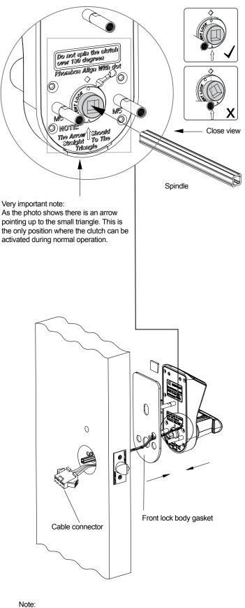
Installing spindle, and front lock body
