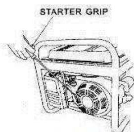
Figure 8 - Pulling the recoil start.
