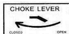
Figure 7 - Choke in the close position
