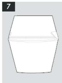
Check that the door is aligned horizontally and vertically and that the seals are closed on all sides before finally tightening the top hinge.
