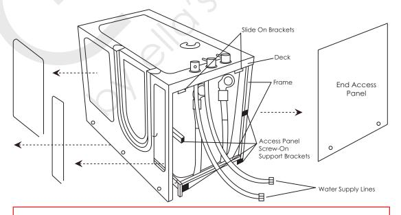
**WARNING:** Lift and carry the tub only by the frame. Protect the bottom of the tub to avoid breaking the air jets positioned on the bottom of the tub.
