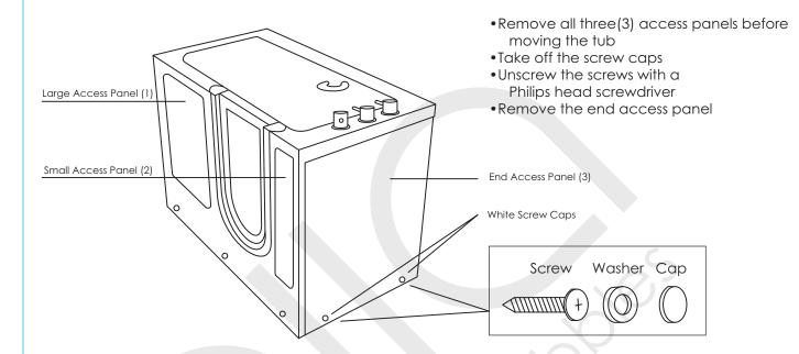
**WARNING:** Do not carry the walk in tub by the panels. Be careful when carrying the tub, avoid front panel contact with the floor or stairs to prevent damages. Make sure no loose parts are hanging down. Remove all three (3) access panels before carrying the tub to prevent them from falling out and breaking.
