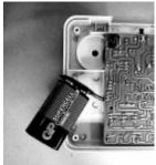
The battery life, (9 volt alkaline battery), is approximately two years if only used for backup.
