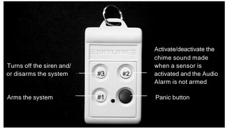
When the Audio Alarm is ON, the four buttons on the transmitter do the following:
