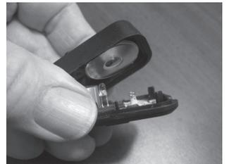
3. Replace battery top with the metal ring visible.
