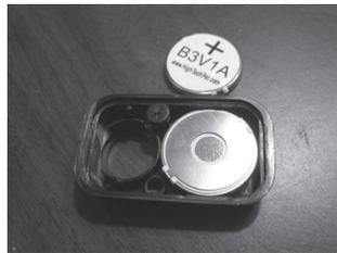
4. Carefully mate top and bottom while keeping aluminum speaker centered in the top hole. Squeeze together the top and bottom until both ends snap.
