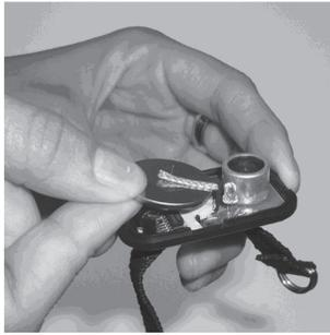
3. To close, first line up the slots at one end of the unit and squeeze together. Then squeeze together on the opposite end until the unit snaps shut.
