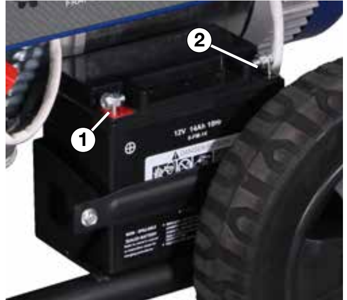
Figure 6 - Attaching the Negative (-) Battery Wire (black)
