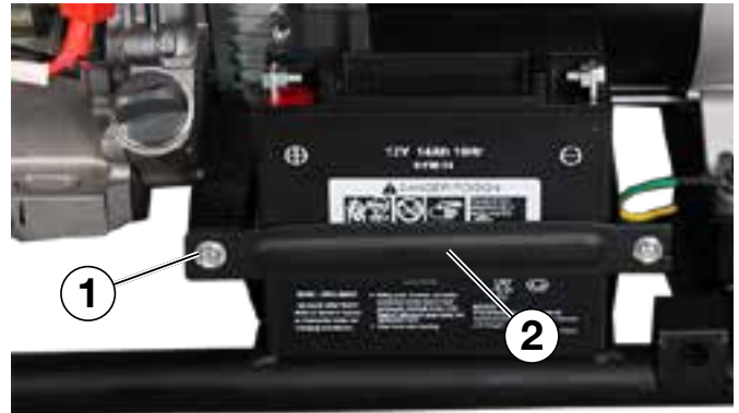
Figure 36 - (1) Bolt, (2) Battery Hold Down Plate
