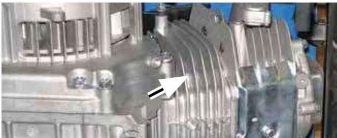
Figure 39 - Engine Cooling Fins
