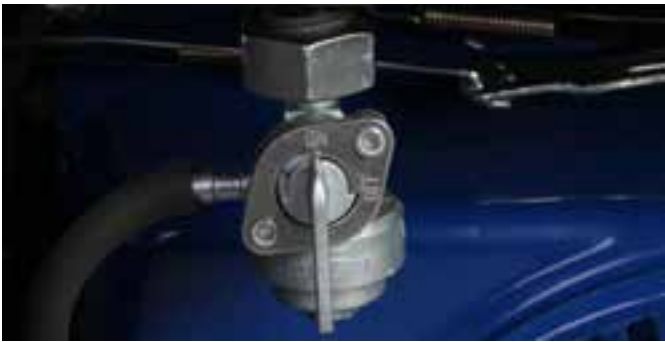
Figure 19 - Fuel Shut Off - ON
