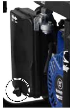
Figure 30 - Some units have a knob at the bottom which secures air filter
