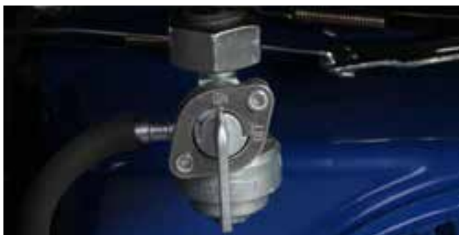
Figure 14 - Fuel Shut Off - ON
