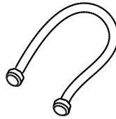
Toilet water supply line
