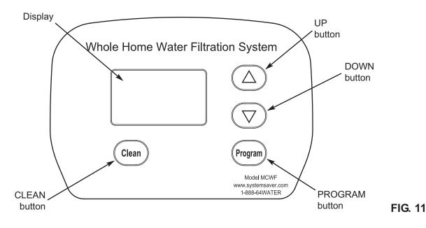
When the transformer is plugged into the electrical outlet, a model code and a test number (example: J1.4), begin to flash in the faceplate display. Then, 12:00 PM and the words "PRESENT TIME" begin to flash.
