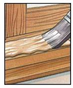
Pour a small amount of the stripper into a convenient glass or metal container, and apply it as specified on the label. It's best to start at the top of your project, and work your way down. Take the time to work it into hard-to-reach places.
