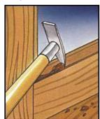
Reapply the stripper to detailed or problem areas, and use specialty scrapers to remove the softened material. Use light pressure on the scrapers to keep from tearing or gouging the wood. If you can't find a contoured scraper, use the corner of a putty knife.
