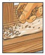
Sprinkle a light coating of sawdust over the stripper just before you remove it. The sawdust thickens the stripper, making it easier to remove.
