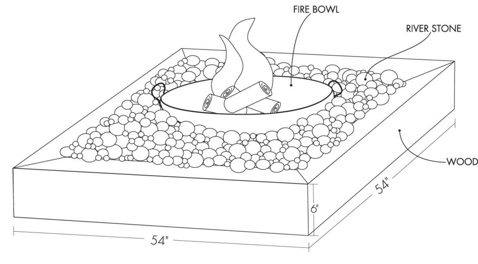
ends so corners conjoin neatly. Screw decorative ledge flush onto support frame with non-rusting galvanized screws. If desired, paint or stain exterior surfaces before proceeding to next step.
