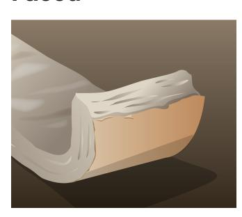
Faced insulation uses kraft paper vapor barriers to control moisture transmission between walls and floors.
