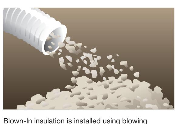
machines; best for adding additional insulation in attic.
