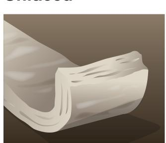
Unfaced insulation does not have a vapor barrier; can be used over existing insulation in the attic, or where moisture control is not needed.
